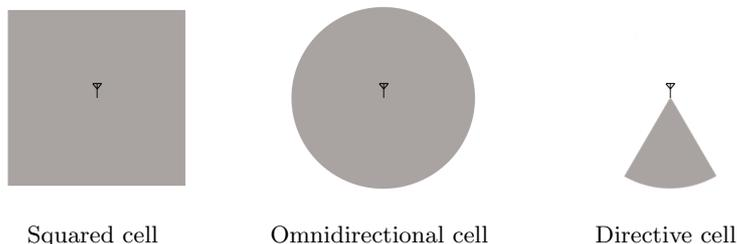
**Fig. 1.** Terrain coverages with different types of antenna
