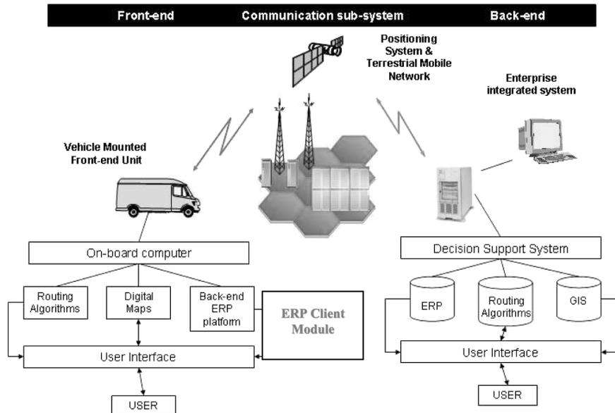
**Figure 3.** Proposed system architecture for real-time vehicle management
