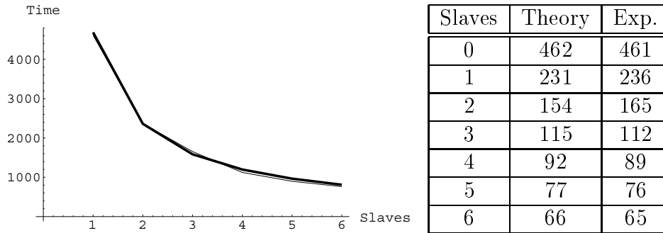
Figure 3.8: Elapsed times (sec) per generation for the NN problem.
