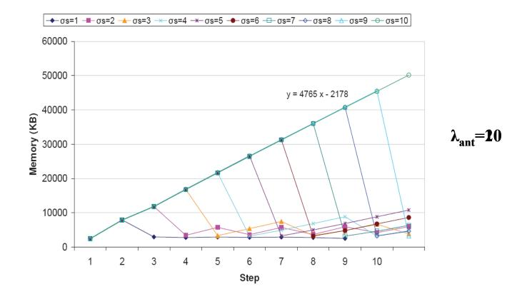
• The pheromone reset after each stage keeps the memory consumption below an upper bound
