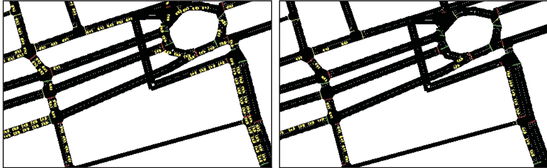
Figure 10.11: Simulation traces of the traffic flow (cars in white) resulting from the cycle programs generated by both, SCPG (left) and PSO (right). The pictures show snapshots at the end of the simulation time. The reader can see that the SCPG leaves a dense traffic while PSO has cleared the routes and the traffic is very fluid and smooth
